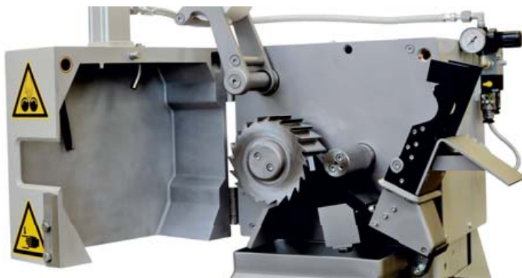
View into the cutting chamber
