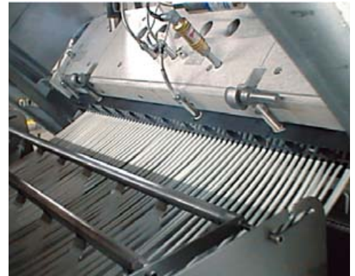
SG 900 die head in operation
