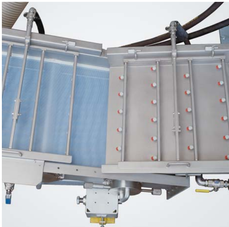
Transition zone of a JSG 600: strand guide section – conveyor
