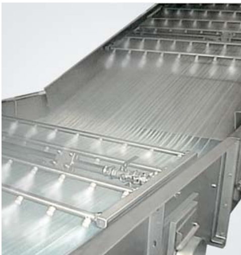
Transition zone from strand guide section to conveyor belt
