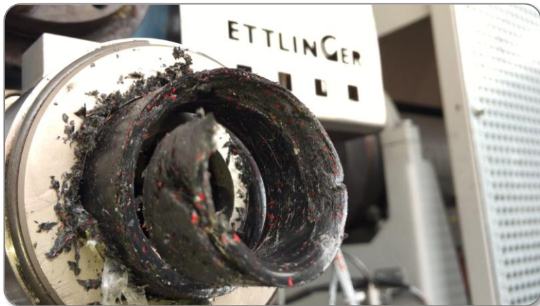
PP Car Bumpers with Paint Contamination
