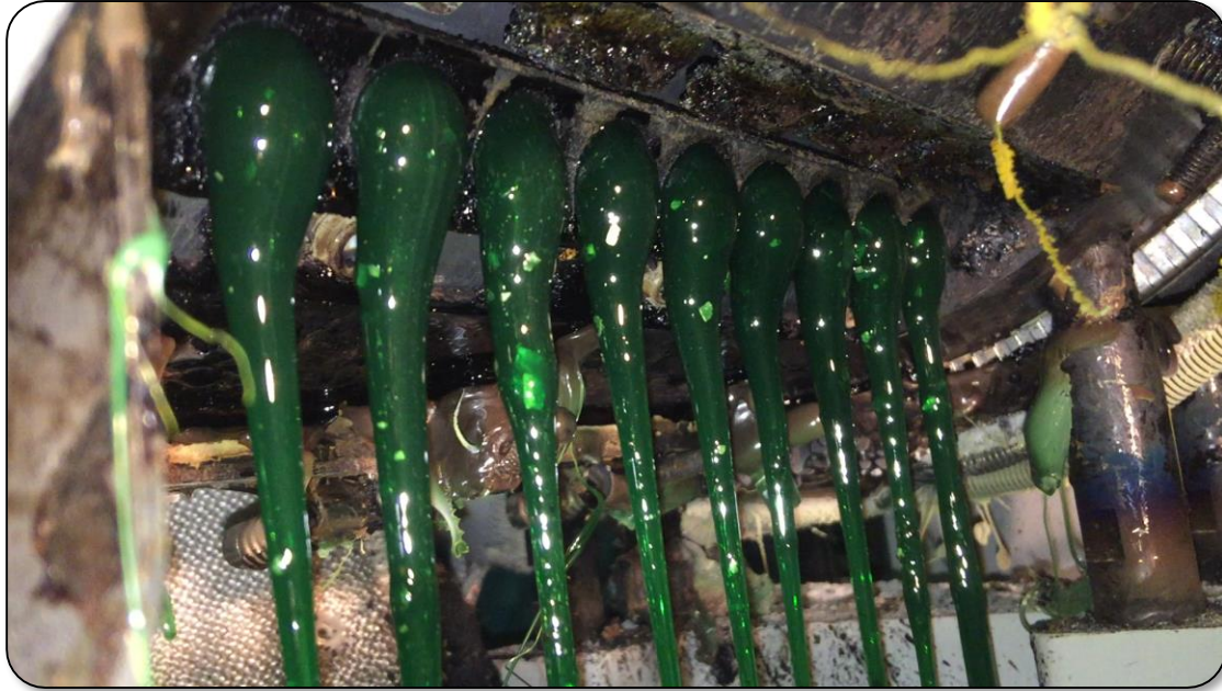
RPET Flake with Aluminum Contamination
