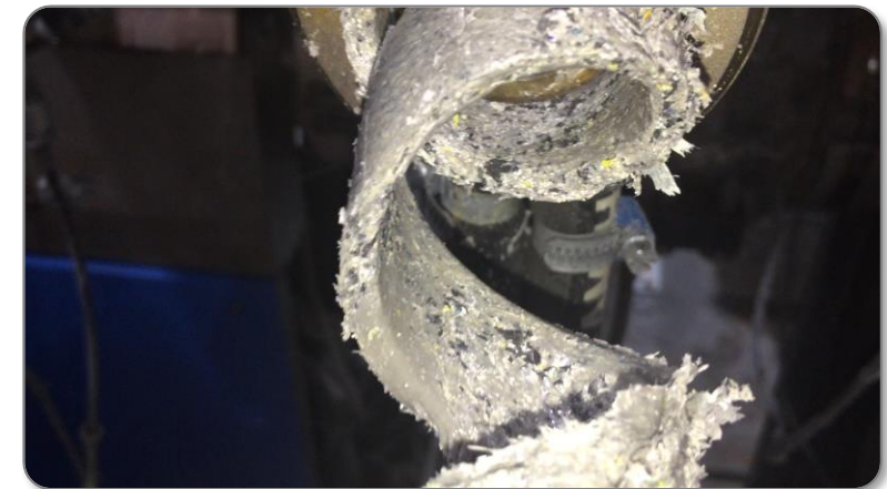
HDPE with Rubber Contamination
