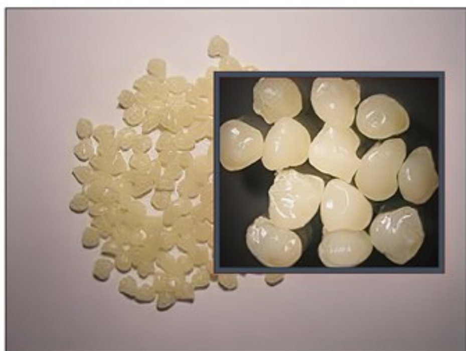
Fewer blades at high cutter speed
