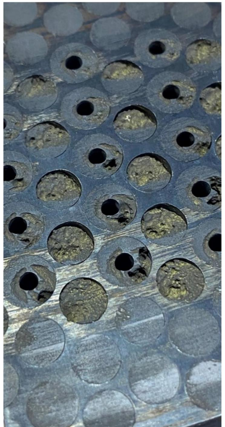
**FIG 1** Acid attack has caused serious damage on the cutting face of this pelletizer. Photos: Maag
