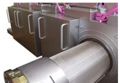
Screen assembly (CSC-R installed for vertical melt flow)
