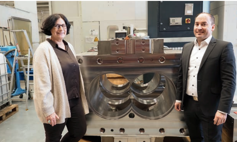
Marketing Manager Iris Fischer and Jonathan Hummer, Head of Product Management Pumps, invite Plastics Insights to tour the Maag Pump Systems AG headquarters in Oberglatt near Zurich, Switzerland. The picture shows the housing of a dual pump for two gear wheel sets.
