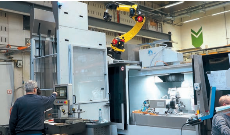
Smaller designs are produced in larger volumes. The machinery is designed to run unmanned shifts in order to handle those demands. Pictured here is a robot serving two milling centers. © Hanser/Schröder
