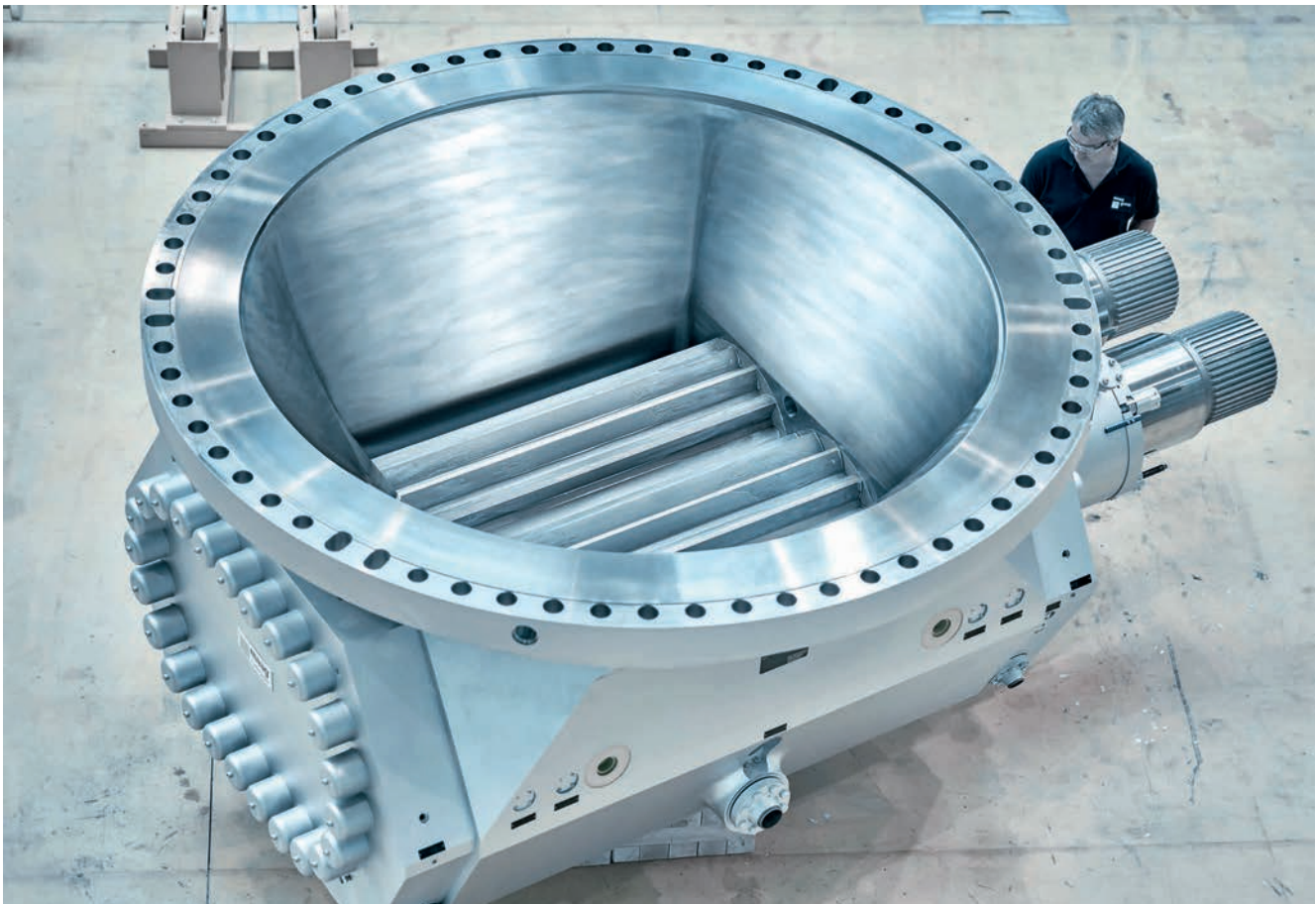
This ultrarex compounding pump holds the company's own record for size: it weighs 48 t, has a pump length of 4 m, and operates at a throughput of 50 t/h. © Maag
